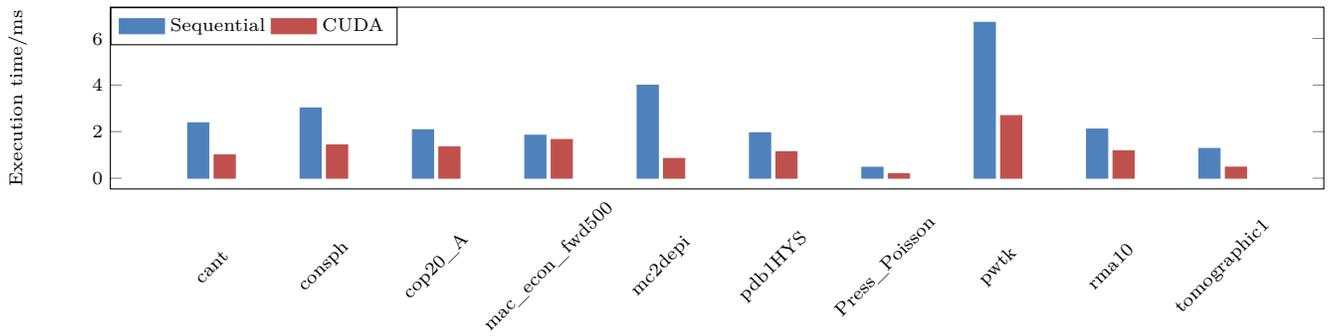
Figure 10: Execution Time comparison between sequential and CUDA CSR SpMV code
